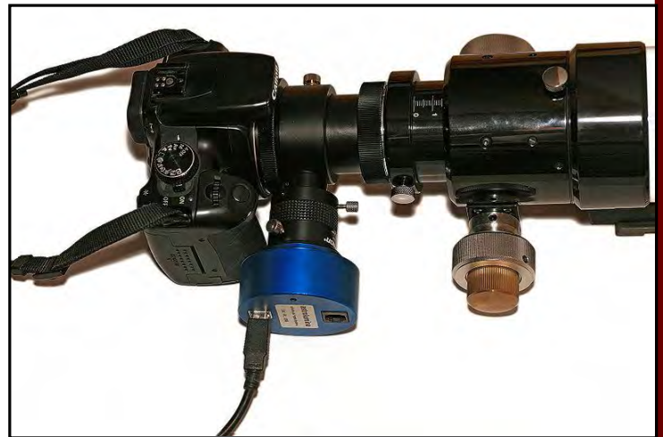
Figure 9. Off-axis guider mounted in front of a DSLR camera. A small prism reflects a star image near the edge of the field of view to the autoguider.
