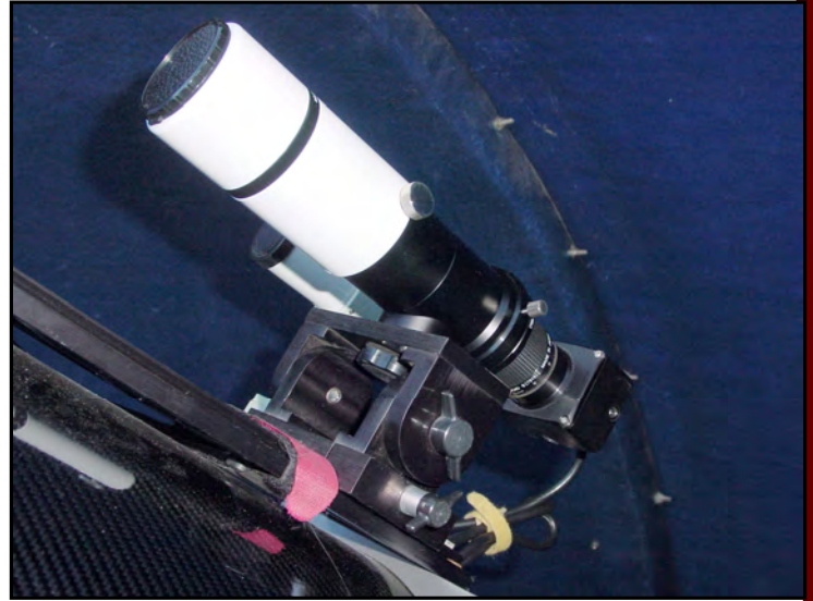
Figure 8. Guide scope and guider mounted on top of a larger imaging telescope.
